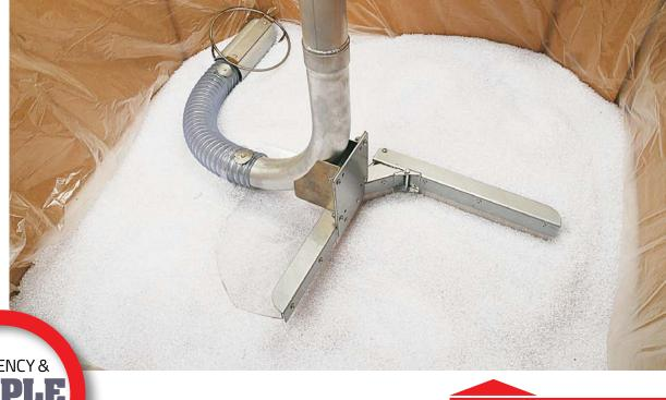
SYSTEM CONSISTENTLY FLATTENS **MATERIAL PILE, PUSHING MATERIAL** TO EDGE OF BOX AND CONVEYED **DIRECTLY**
