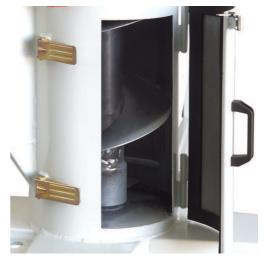
Detail of the inspection door of the mixing screw.
